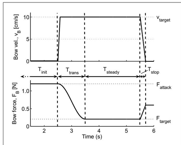
Figure 1. An example of bow velocity and bow force contours used for measuring Schelleng diagrams. The acceleration-force combination during the attacks (start of  $T_{trans}$ ) was chosen to obtain short pre-Helmholtz transients. During the transition phase  $T_{trans}$  the force was smoothly changed to the target force  $F_{target}$ . Bow velocity and bow force were kept constant during  $T_{steady}$ .
