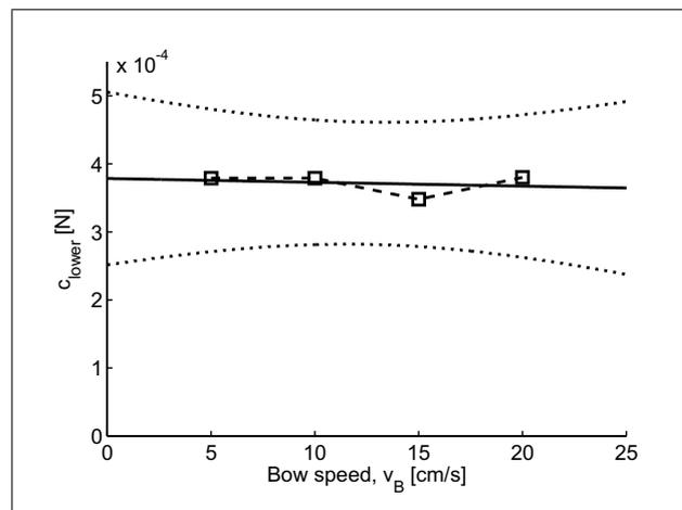
Figure 10. Mean values of  $c_{lower}$  versus bow velocity for the D string in Experiment II. The best linear fit (solid line) and the 95% prediction interval (dotted lines) indicate that the minimum bow-force limit was not dependent on bow velocity within the measured range 5-20 cm/s.
