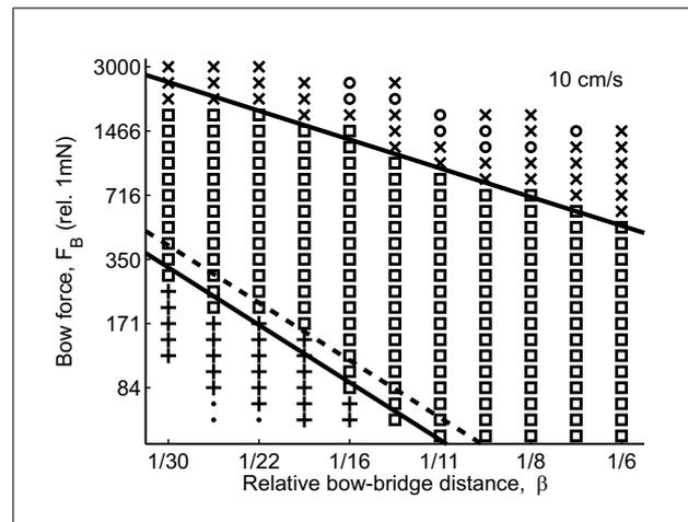
Figure 6. Reproduced Schelleng diagram at a bow velocity of 10 cm/s, measured about 5 months earlier than the corresponding diagram in Figure 4 (b). The solid lines represent the fitted Schelleng limits. The dashed line indicates the fitted lower bow-force limit in Figure 4 (b). The fitted upper bow-force limits coincided exactly.
