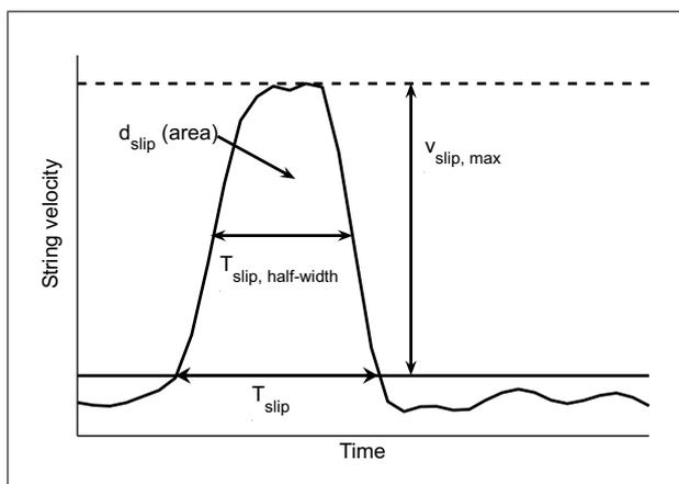
Figure 12. Features used to characterize the shape of the slip phase: the traversed distance during slip (area of the slip phase,  $d_{slip}$ ), the maximum slip velocity  $v_{slip,max}$ , the duration of the slip phase  $T_{slip}$  and the width of the slip phase at half height  $T_{slip,half-width}$ .
