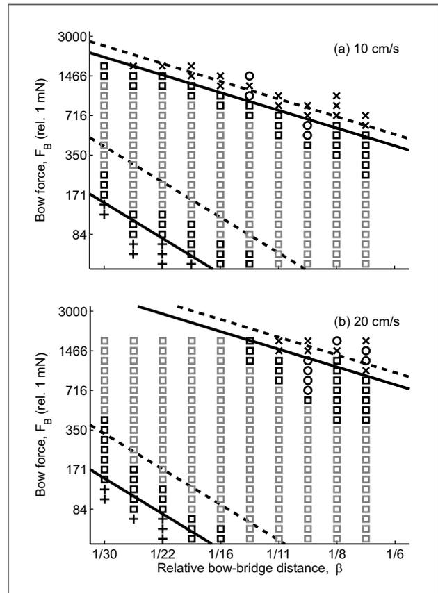
Figure 7. Schelleng diagrams for a steel E string mounted on a monochord at bow velocities (a) 10 and (b) 20 cm/s. The fitted Schelleng limits are indicated with solid lines. The fitted bow-force limits of the D string in Figure 4 are indicated with dashed lines. The middle parts of the Helmholtz regions, indicated by gray squares, were not systematically analyzed, but there was no doubt about the consistency of Helmholtz motion.
