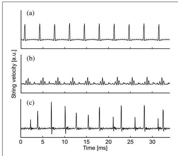
Figure 2. Examples of common types of string motion (velocity) as recorded in the experiments: (a) Helmholtz motion, (b) multiple slipping and (c) raucous motion.
