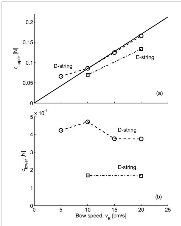
Figure 8. Dependence of the bow-force limits on bow velocity in Experiment I. The plots show (a)  $c_{upper}$  and (b)  $c_{lower}$  as function of bow velocity, estimated from the Schelleng diagrams of the D string (circles) and E string (squares). According to the Schelleng equations there should be a linear relationship. The solid line in (a) shows a least-squares fit of the upper bow-force limit of the D string according to equation (1), under the assumption that  $\Delta\mu$  is constant.
