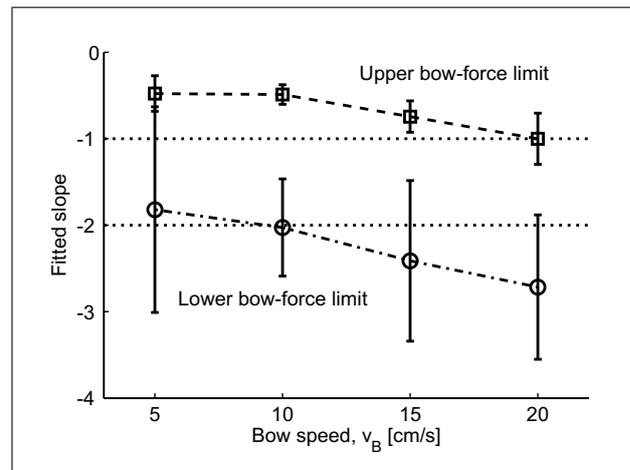
Figure 5. Fitted slopes of the upper bow-force limits (squares, dashed line) and the lower limits (circles, dash-dotted line) in the Schelleng diagrams for different bow velocities in Figure 4. The error bars indicate the 95% confidence intervals of the fitted values. The predicted slopes for maximum and minimum bow force ( $-1$  and  $-2$ ) are indicated by the horizontal dotted lines.
