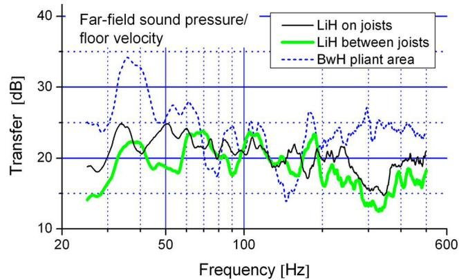
FIG. 4. (Color online) Transfer functions from stage floor to sound in the hall for LiH and BwH calculated as sound pressure/stage-floor velocity averaged over six positions in the audience area (LiH on joists, thin line; LiH between joists, thick line; BwH in pliant area, dashed line). Sound pressure is relative to 94 dB SPL, while other parameters are relative to ISO standard units.
