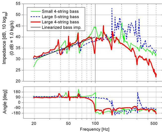
FIG. 7. (Color online) Input impedances measured at the end pin of three double basses. All basses show phase values of approximately  $90^\circ$  in the region 20–80 Hz. In the same interval the average impedance is rising approximately 4 dB/octave. Small four-string bass (thin line), large four-string bass (thick line), and large five-string bass (dashed line). The thin straight line indicates a linearized average.
