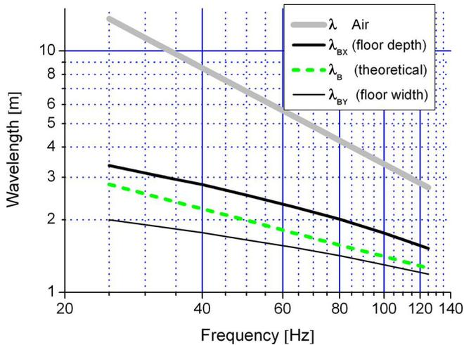
FIG. 3. (Color online) Measured bending wavelengths of the LiH floor in two directions, compared to wavelengths in the air (thick line) and to the rule of thumb, Eq. (1) (dashed line).
