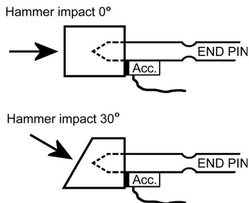
FIG. 6. Adapters mounted to the double-bass end pins facilitating clean force-hammer impacts at two angles (0° and 30°).
