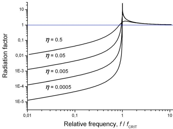
FIG. 5. (Color online) Radiation factors of an infinite plate with losses (indicated by loss factor  $\eta$ , see the text). Adapted from Ref. 13.
