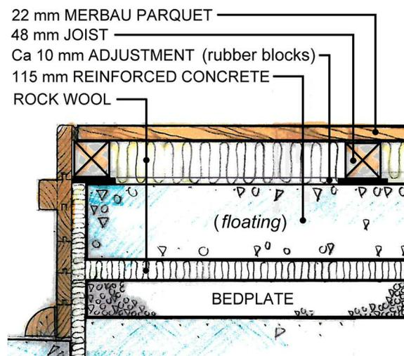
FIG. 1. (Color online) Stage-floor construction in LiH. The joists, only 30 cm apart, are resting on floating, reinforced concrete, with thin rubber blocks in between. (Drawing made available by courtesy of Arkitektgruppen Lille Frøen AS.)
