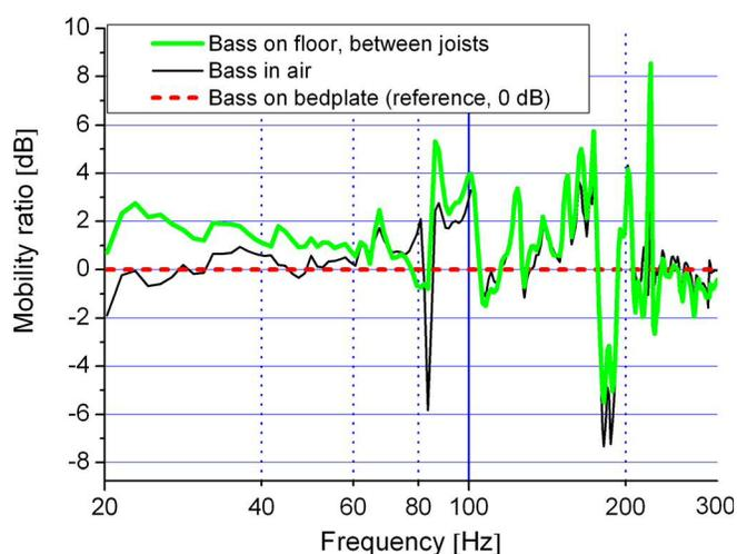
FIG. 9. (Color online) Changes in bridge mobility caused by the support of the end pin. The foundation under the end pin plays an important role for the playability of the double bass through the impact on the bridge mobility. Bridge mobility of a large five-string bass in LiH, measured with the end pin resting on rigid bedplate (0 dB reference); on the stage floor between joists (thick line), and bass suspended in the air (thin line).
