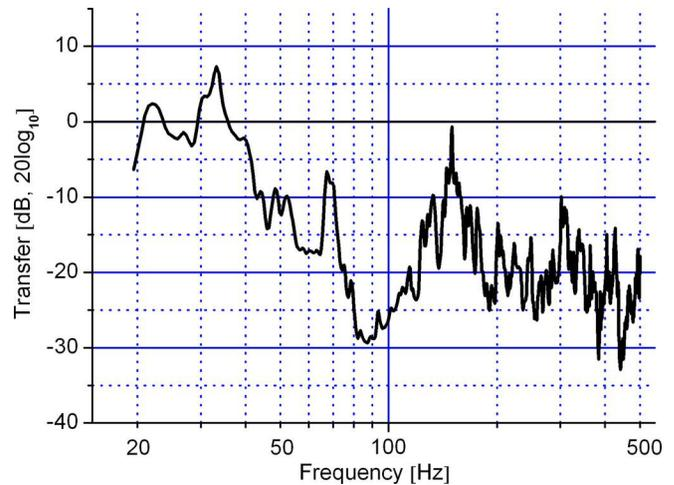
FIG. 8. (Color online) Vibration velocity transfer from the double-bass bridge to the floor adjacent to the end pin (five-string bass in pliant area of BwH).
