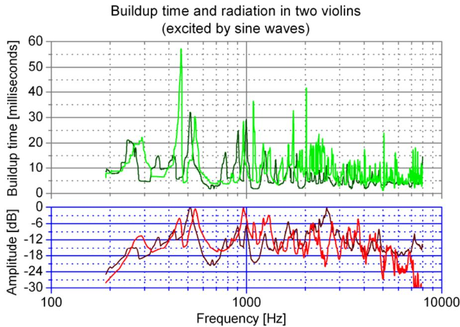
**Figure 1:** Buildup time compared to radiation (sound pressure) of two violins: dark colors for a Francesco Ruggeri; light colors for an Antonio Stradivari. Notice how the long-lasting transients correspond with major resonances of the violin body. The longer buildup time above 1000 Hz for the Stradivarius is mainly due to the measuring technique (see text).
