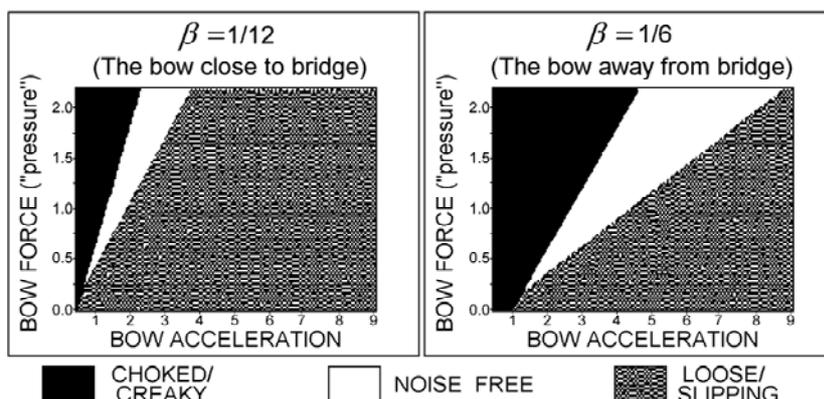
**Figure 4:** The “clean-attack”/“noise-free” delta gets smaller as the bow is moved towards the bridge. Greater bowing precision is needed to control the attack near the bridge, where the acceleration must be kept steady and low.
