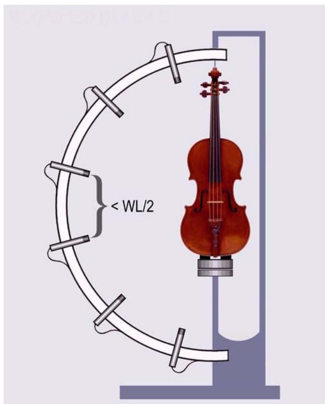
**Figure 11:** Setup for radiation measurement in an anechoic room. By placing a microphone array in a semicircle, the radiation of an instrument (rotated in steps) can be estimated at all angles. The distance between individual microphones should preferably be less than half the wavelength of the highest frequency where separation of individual modes is desired.
