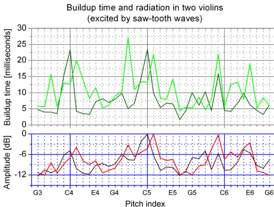
**Figure 2:** Buildup time compared to radiation of a violin when the input signal is a saw-tooth wave, as comparable to loud playing. Notice that the radiation amplitude is more even now than it was with the pure sine-wave input signal. Also: buildup-time is somewhat shorter in the low-frequency end. Only tones of the chromatic scale were recorded.
