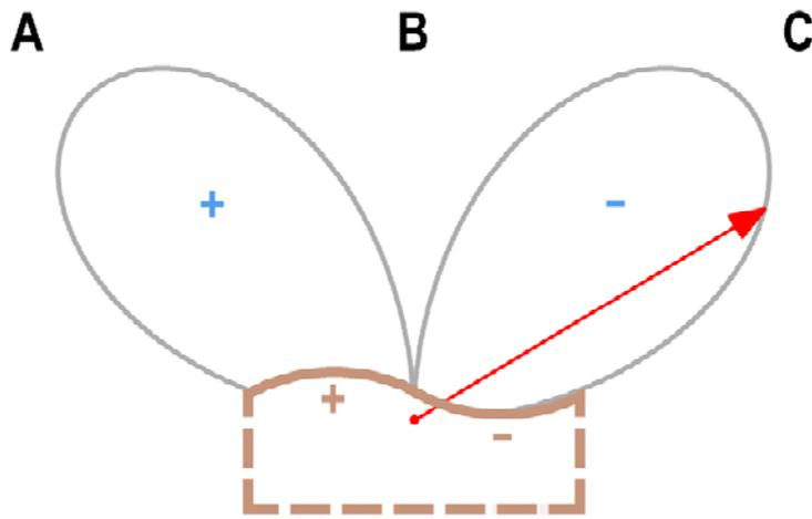
**Figure 9:** Example of multipole sound-pressure in the near field. While the left side of the box is creating *increased* air pressure on its outside, the situation is opposite on the right side where air is sucked in. The red arrow is indicating the relative pressure magnitude at the different angles. Notice that while microphone positions **A** and **C** both will record maximum sound pressure at that distance, position **B** will record no sound for this particular frequency.
