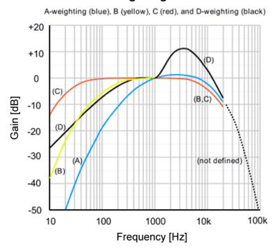
The rationale behind having different weighting curves is that the relative sensitivity of the ear varies with sound intensity as well as with signal characteristics. E.g., dB(A) is best suited for low-level sounds (like noise in audio amplifiers, etc), while dB(C) is best suited for high-level sounds.
